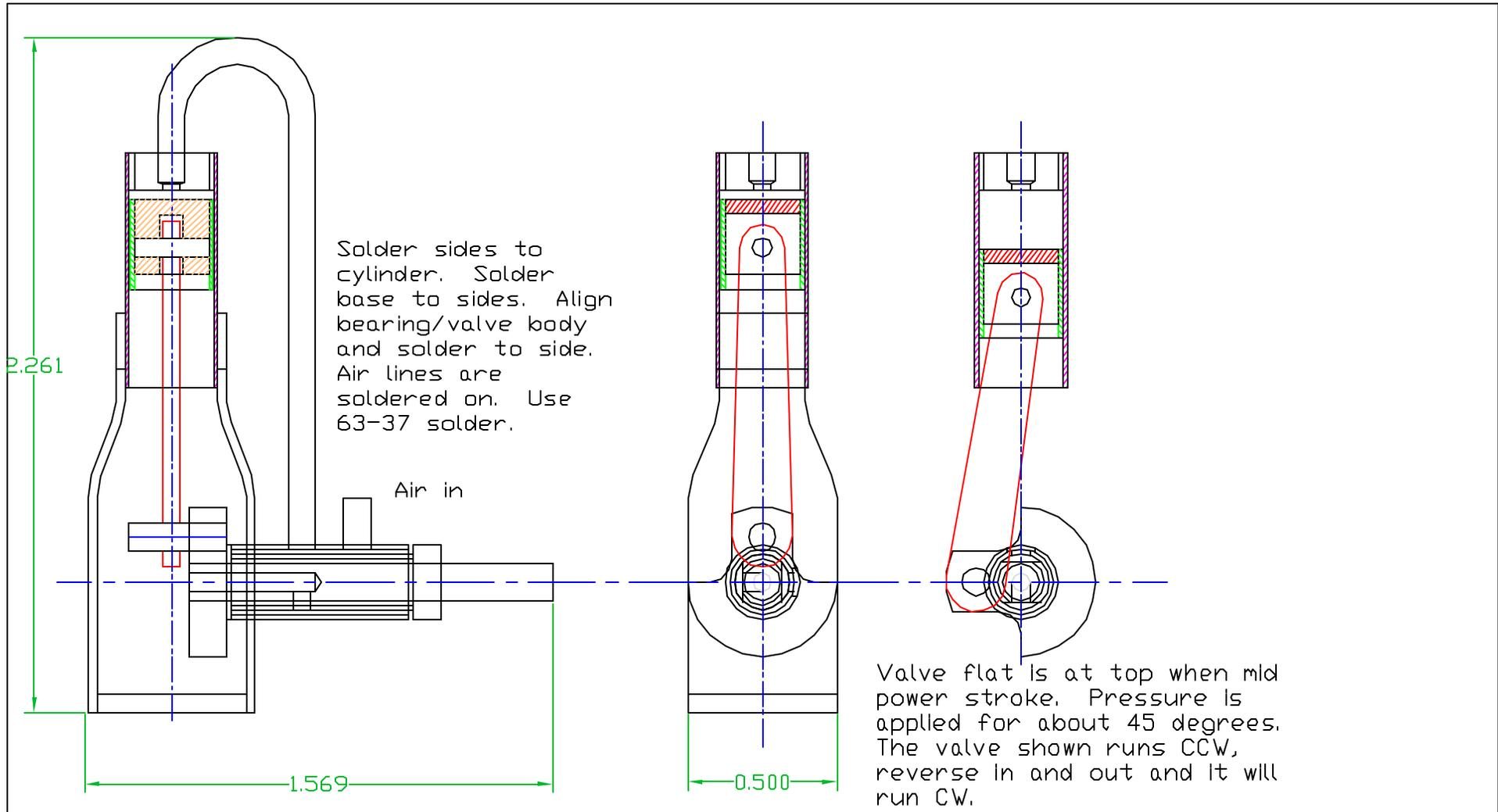
Tube engine is built out of standard hobby shop tubing and hardware store items. The design requires no lathe or mill but they may help improve the appearance.
