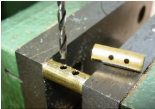
The outer valve body is 2 layers of tube. The inner one is drilled 1/16 and the outer one id driller #41 (.096) to accept the OD of the copper tube to be soldered to it. They get soldered together
