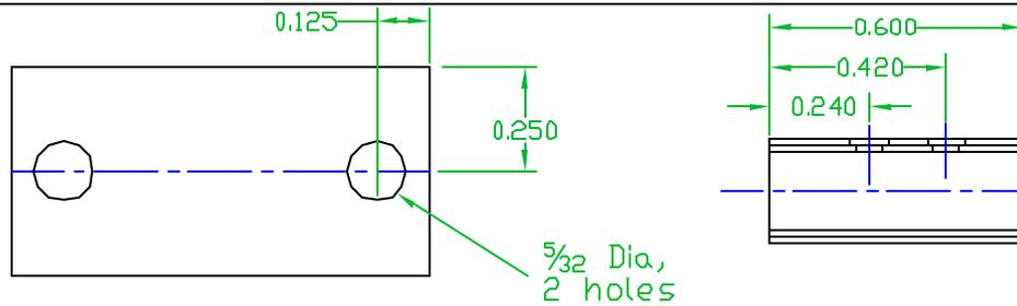
Valve body is a section of  $\frac{7}{32}$  OD Brass tube inside of  $\frac{1}{4}$  OD Brass tube. Side holes are drilled  $\frac{1}{16}$ , then outer tube has holes enlarged to #41 (.096) for  $\frac{3}{32}$  tube. Holes are aligned and tubes are soldered together with half hard solder. Air lines are soft soldered into holes.
