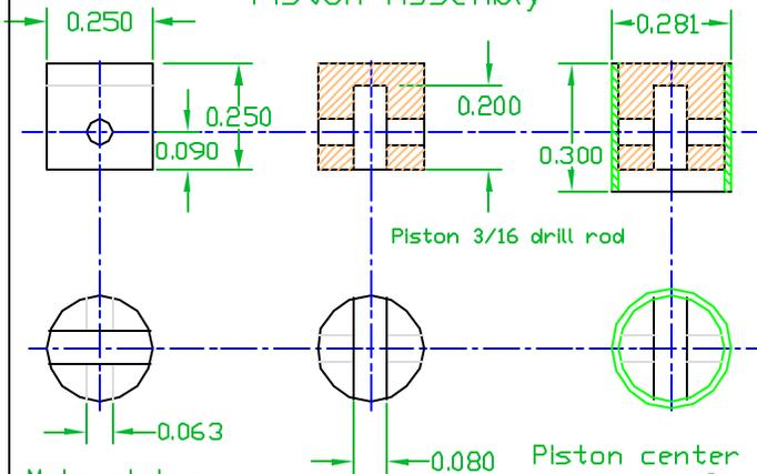
Make piston center from 1/4 aluminum rod. Saw slot, drill wrist pin perpendicular to slot.
