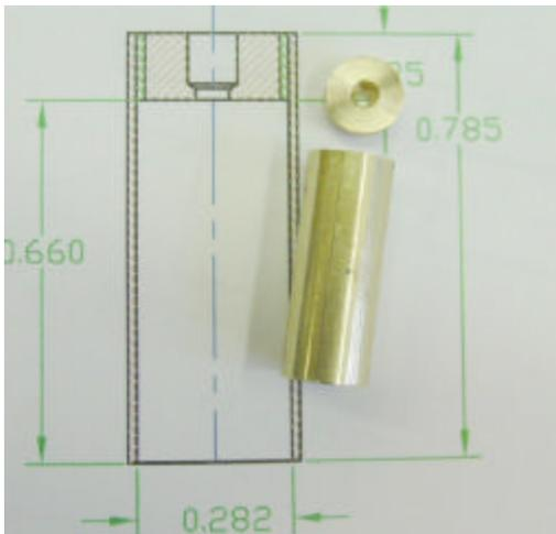
The cylinder is a tube with an end cap made to accept the copper tubes.
