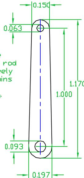
Make sure connecting rod moves freely on both pins before assembling.
