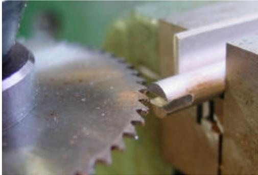
Cut the slot in the piston rod.
