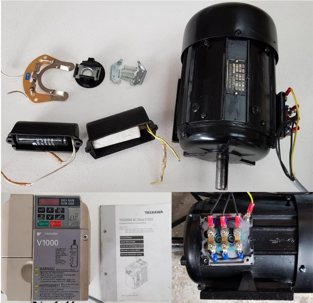
Top – All the single phase starting gear removed.
