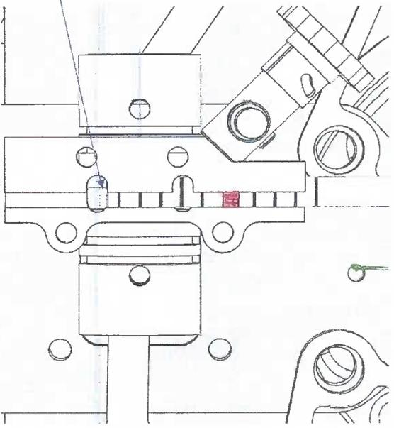
At 173 Deg. Rotation the POWER & PUMP pistons are at their closest point & on LH side, the EXHAUST port is still open. The Power piston is still drifting slowly to the LH, and is the PUMP piston.
