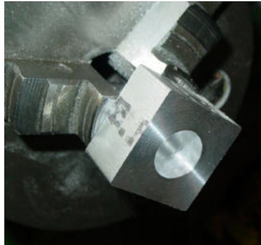
Turn to correct diameter and depth holding bearing boss to improve concentricity. Use light cuts so it will not slip.
