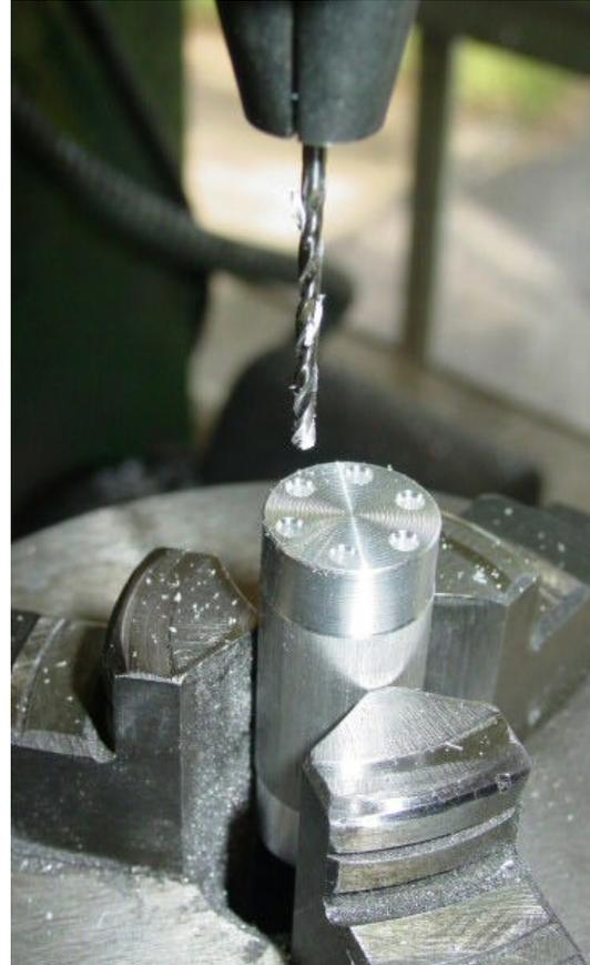
Drill bolt holes in head.
