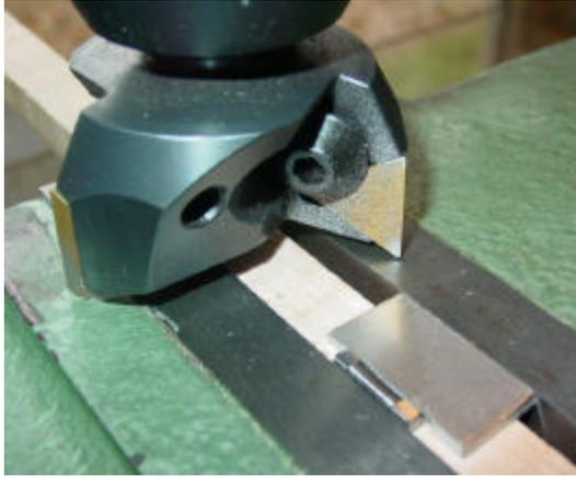
Mill flat sides on connecting rod.
