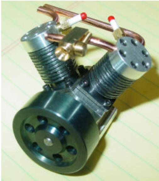
Finally it is complete. With the throttle, plugs and exhaust pipes. It runs great and has a different sound with the V timing.
