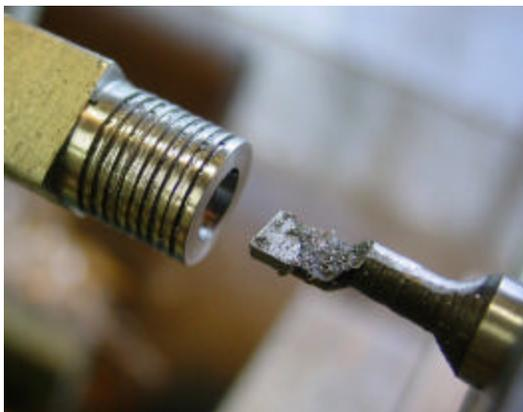
Fins were cut with a slitting saw blade held like a cutter. The bore was drilled slightly undersize. Counter bore was added for the valve disk. The inside was honed with 400 grit lapping compound until a section of  $\frac{1}{4}$  drill fit in, then that was lapped to perfect fit.
