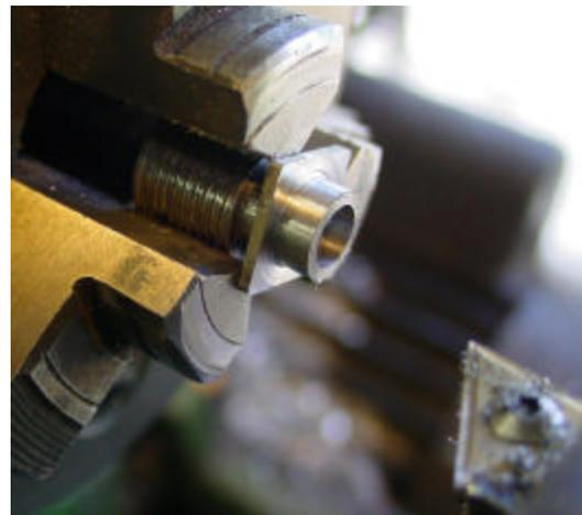
Keep inside flange long to hold in chuck while drilling head and exhaust holes. Turn to length later. The ID needs a champher for connecting rod clearance.
