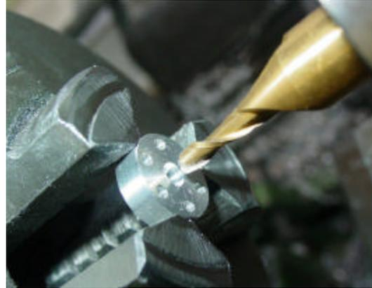
Machine pocket for ball wit 1/8 dia ball cutter. Drill the side ports.
