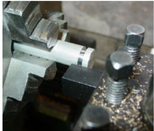
Tube bender, turn a groove the size of the copper tube to bend and move the end of a tool up to the groove.
