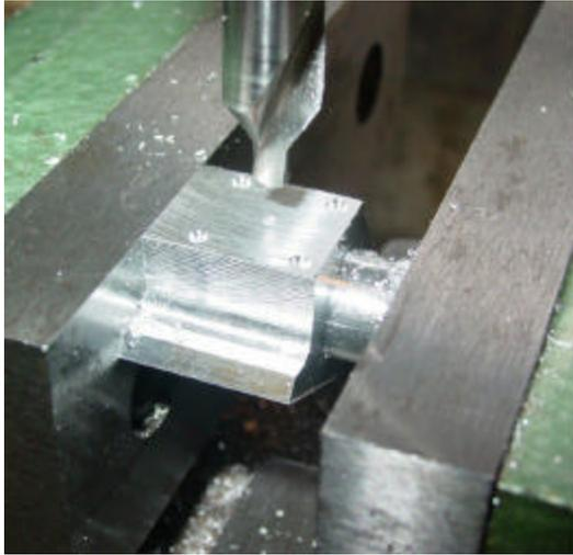
Center drill. Use a large one the start the cylinder holes.
