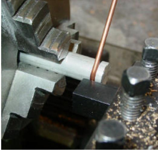
The tool supports the tube, just bend it to the required angle. I adjusted the length on a belt sander.
