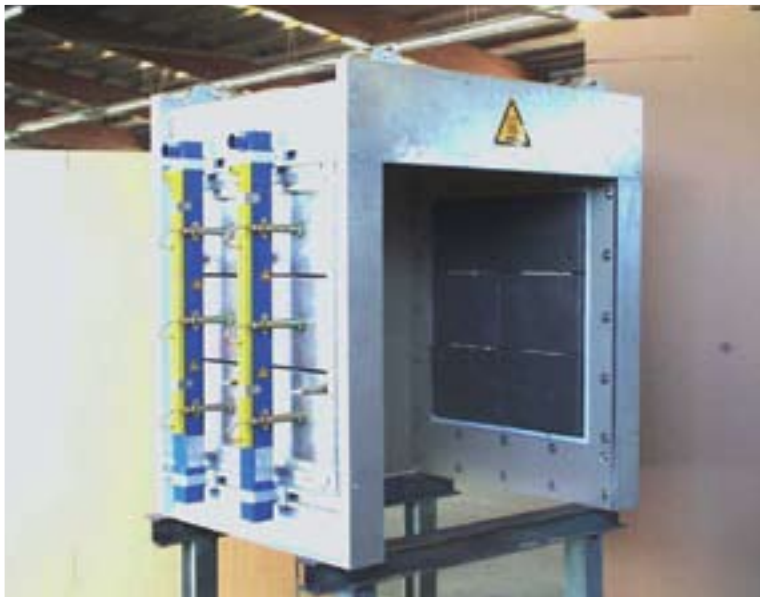
Heating tunnel with GoGaS metal fibre burners
