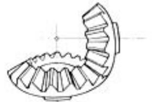
Fig. 2-14 Straight Bevel Gear
