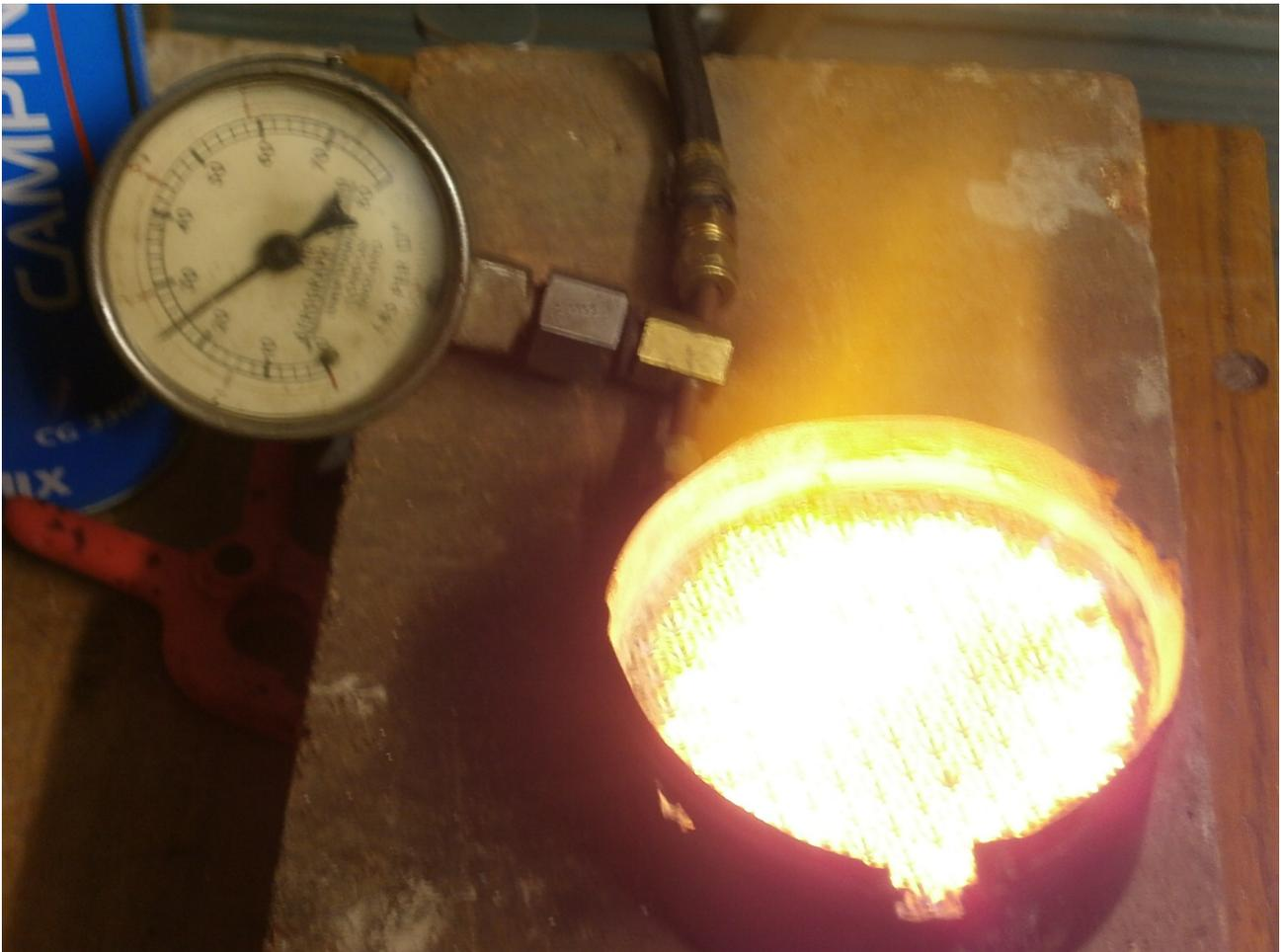
But that is too much for the burner. But as it is designed for 15psi butane it actually works OK with 15psi mixture.
