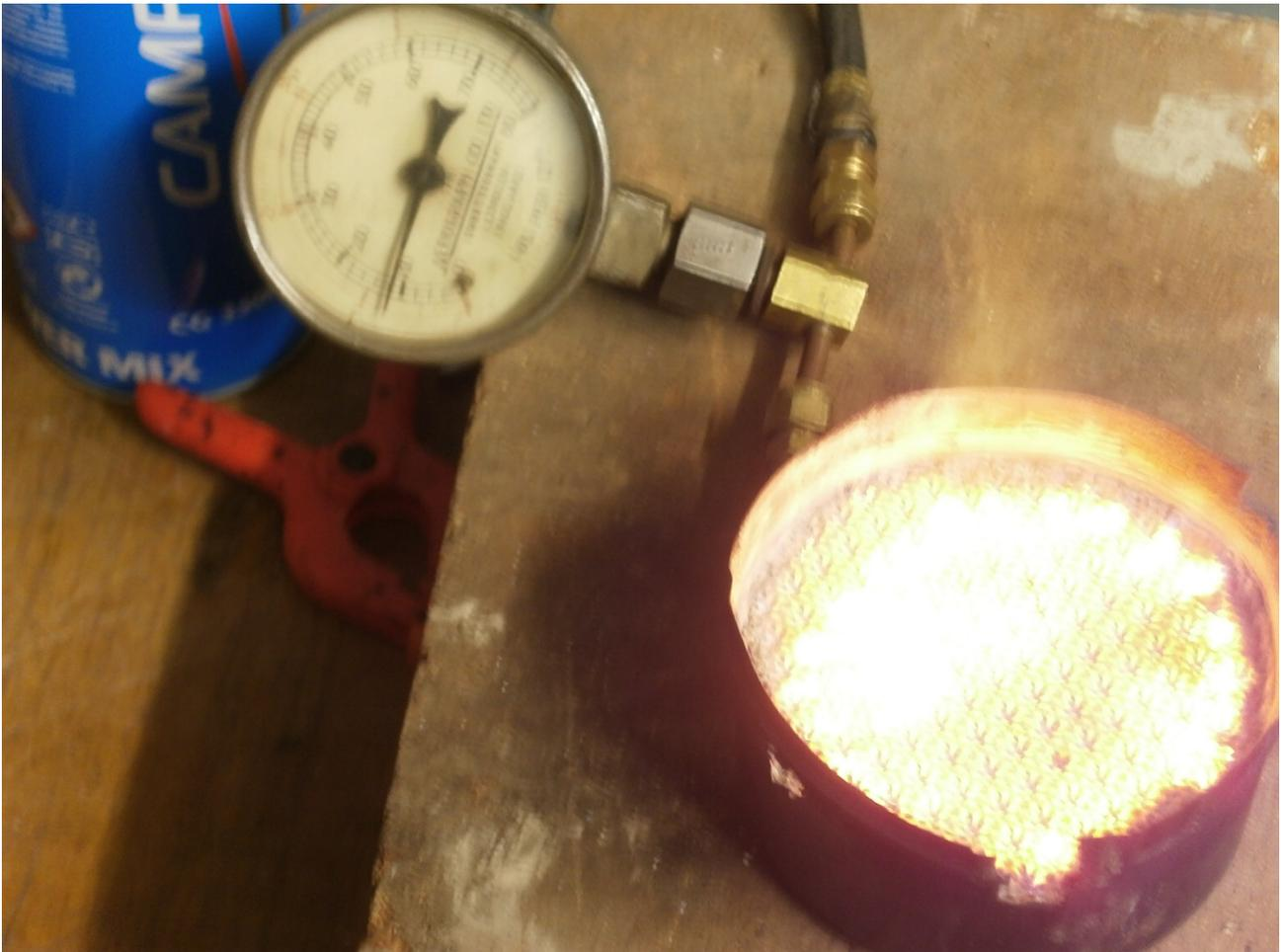
So I reckon on Propane, you'll be OK at somewhere between 10 and 20 psi max. The burner has a no 8 jet, 0.25mm drilling. The mixer tube is 8mm (5/16" ) bore, with 2 x 6mm air holes.
