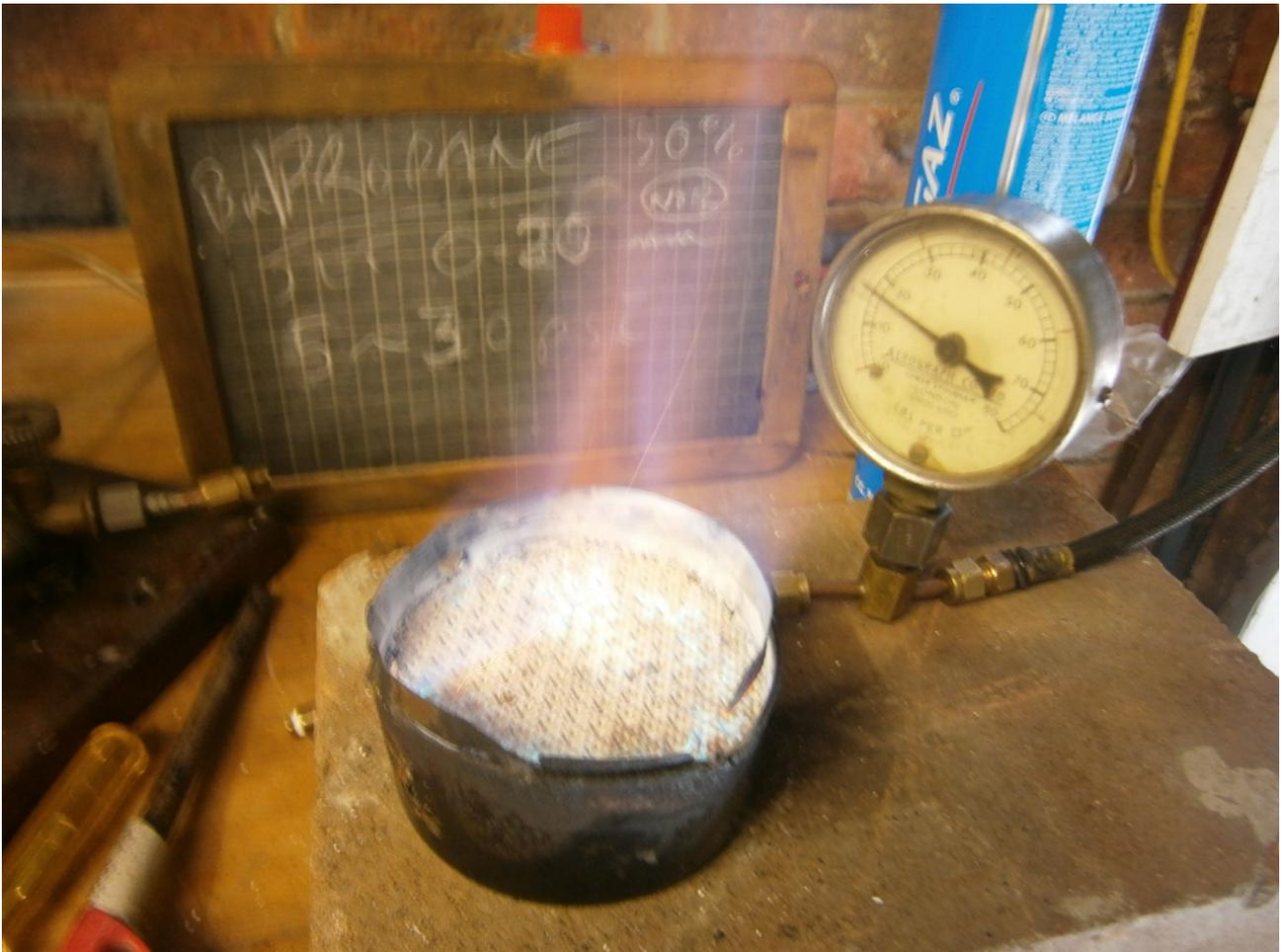
**Conclusion:** With this design of 3inch round ceramic burner, The jet should not exceed 0.25mm (No.8) with the 8mm (5/16 in.) bore mixer and diffuser tube. With Butane, or 70% Butane-30% Propane mixture, the pressure applied shall not exceed 15psi.
