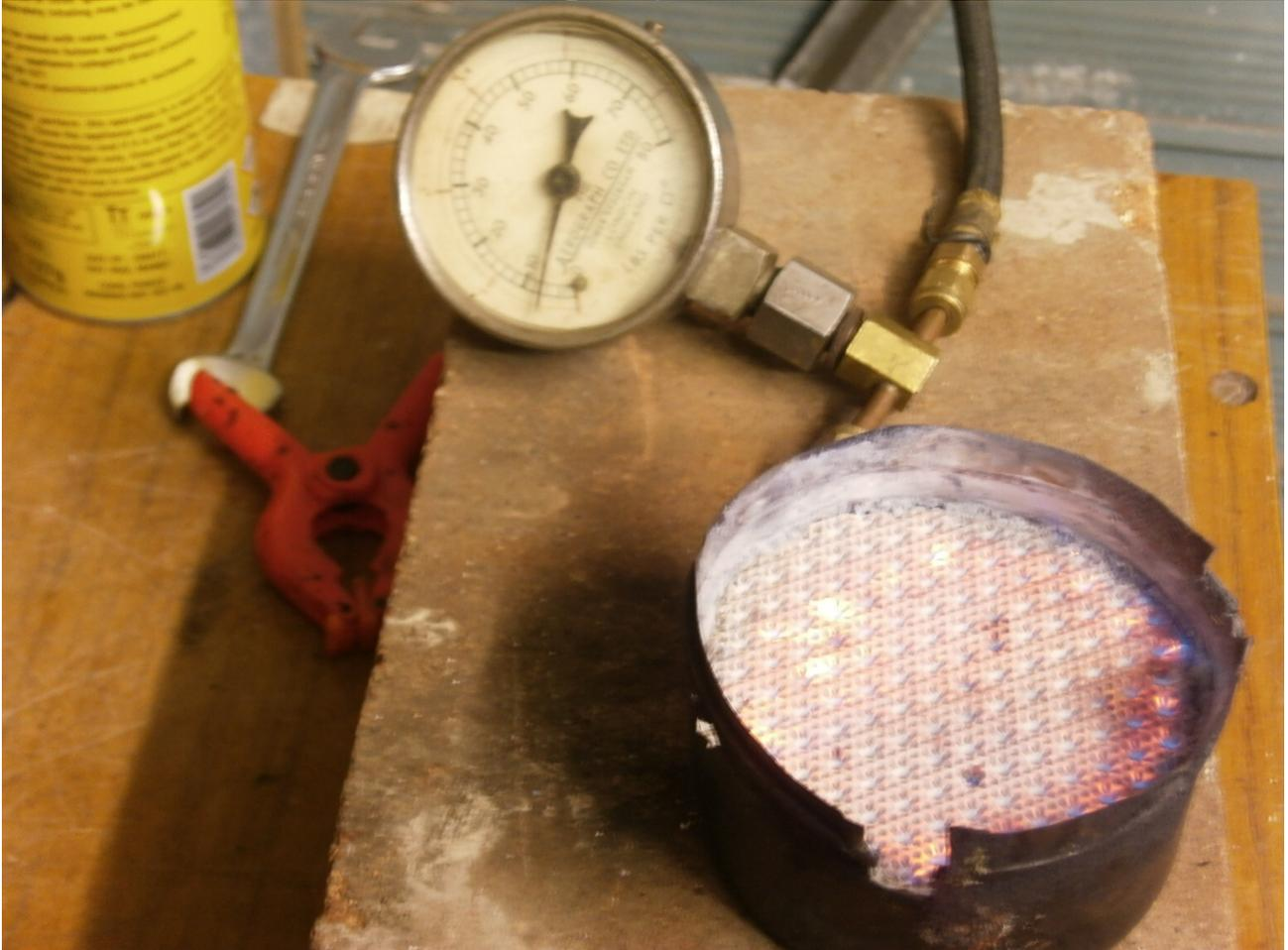
With butane-propane 30%mix, the canister can hold 28 psi max.
