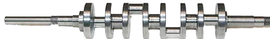
Finished except for cross-drilled oil feed holes
