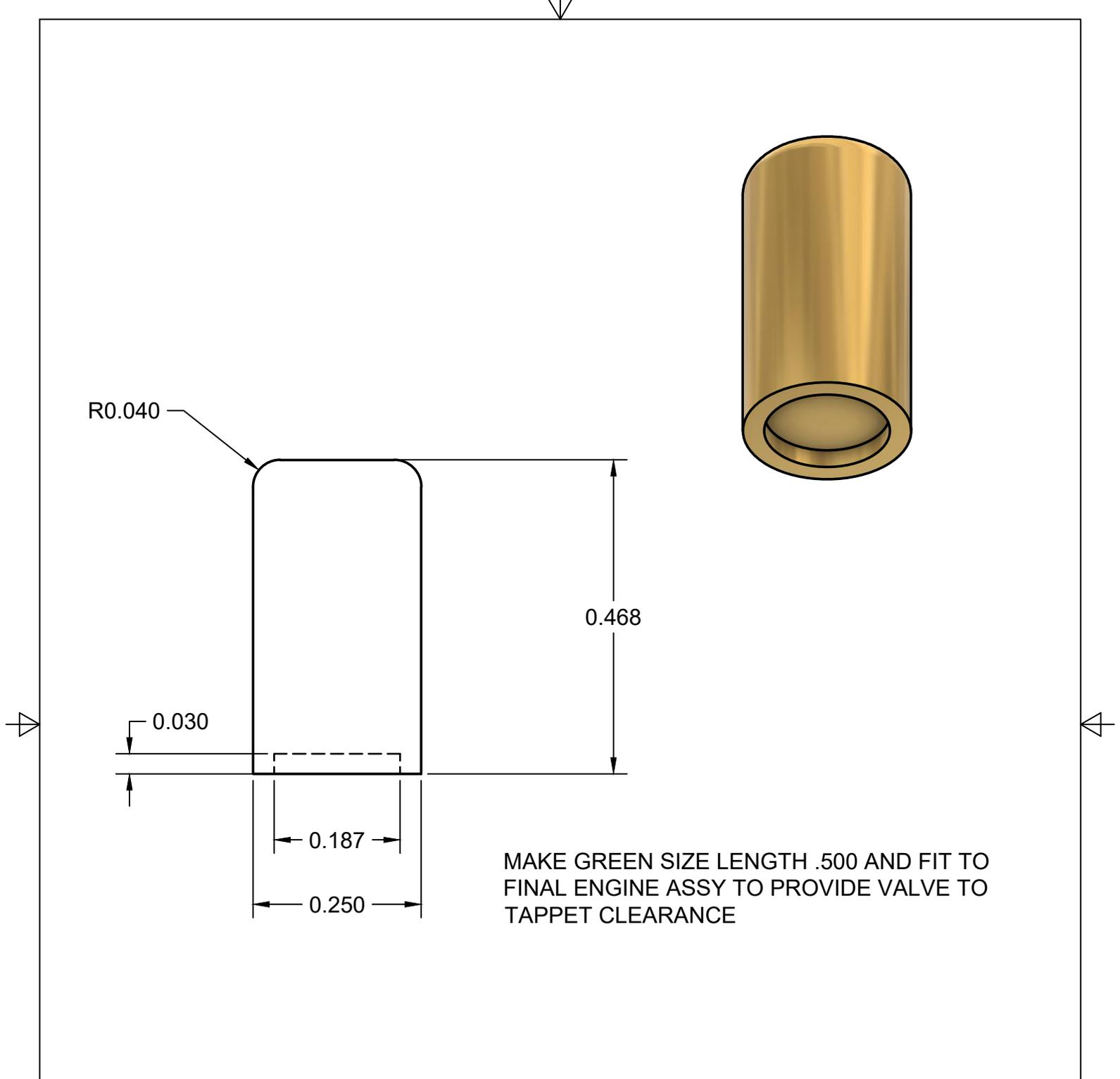
MAKE GREEN SIZE LENGTH .500 AND FIT TO FINAL ENGINE ASSY TO PROVIDE VALVE TO TAPPET CLEARANCE
