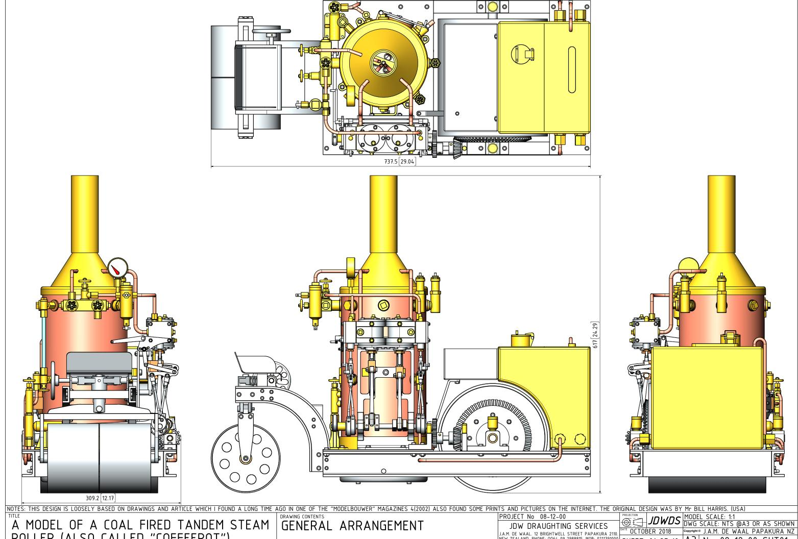
A MODEL OF A COAL FIRED TANDEM STEAM ROLLER (ALSO CALLED "COFFEEPOT")
