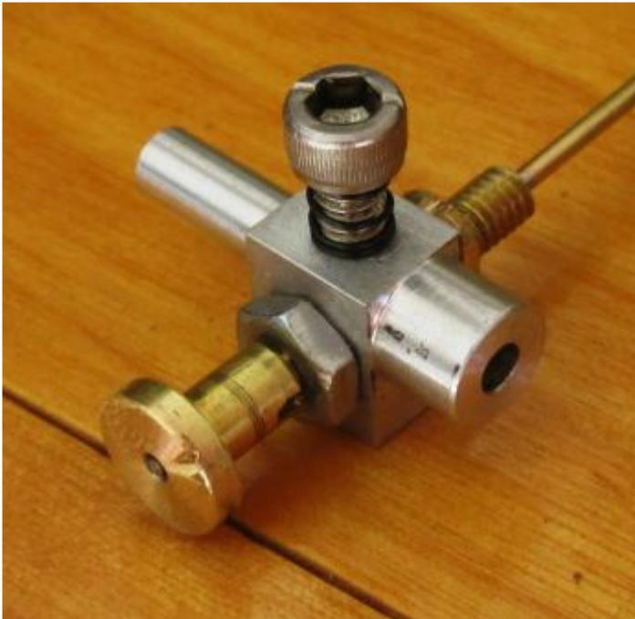
The carburetor body is made 1.5" x 0.5" x 0.375" brass or aluminum. Length may vary depending on application.
