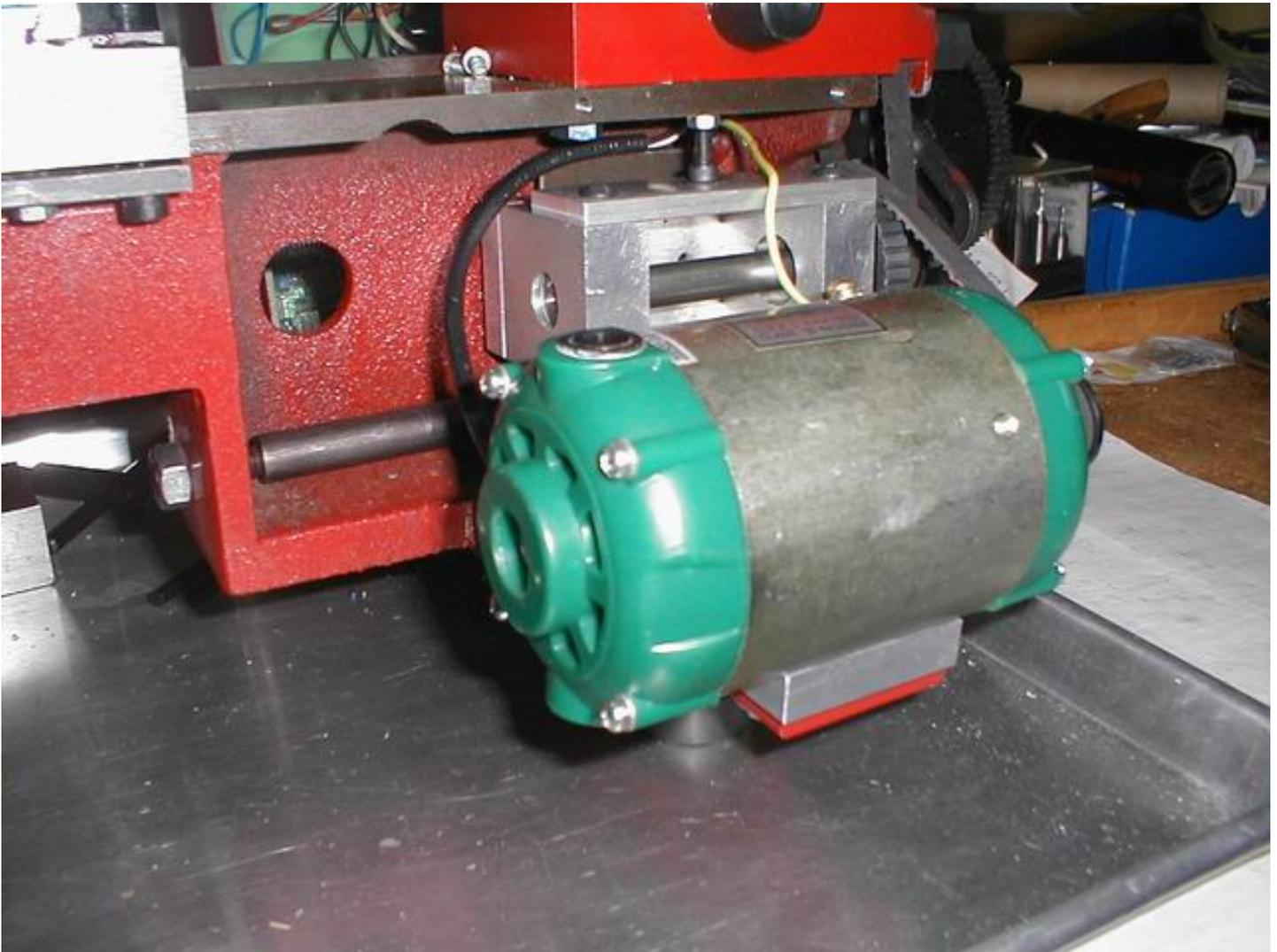
two hex nuts under the mount with a 10mm open end wrench. In this view, the clumsy position of the underside motor brush holder can be seen.
