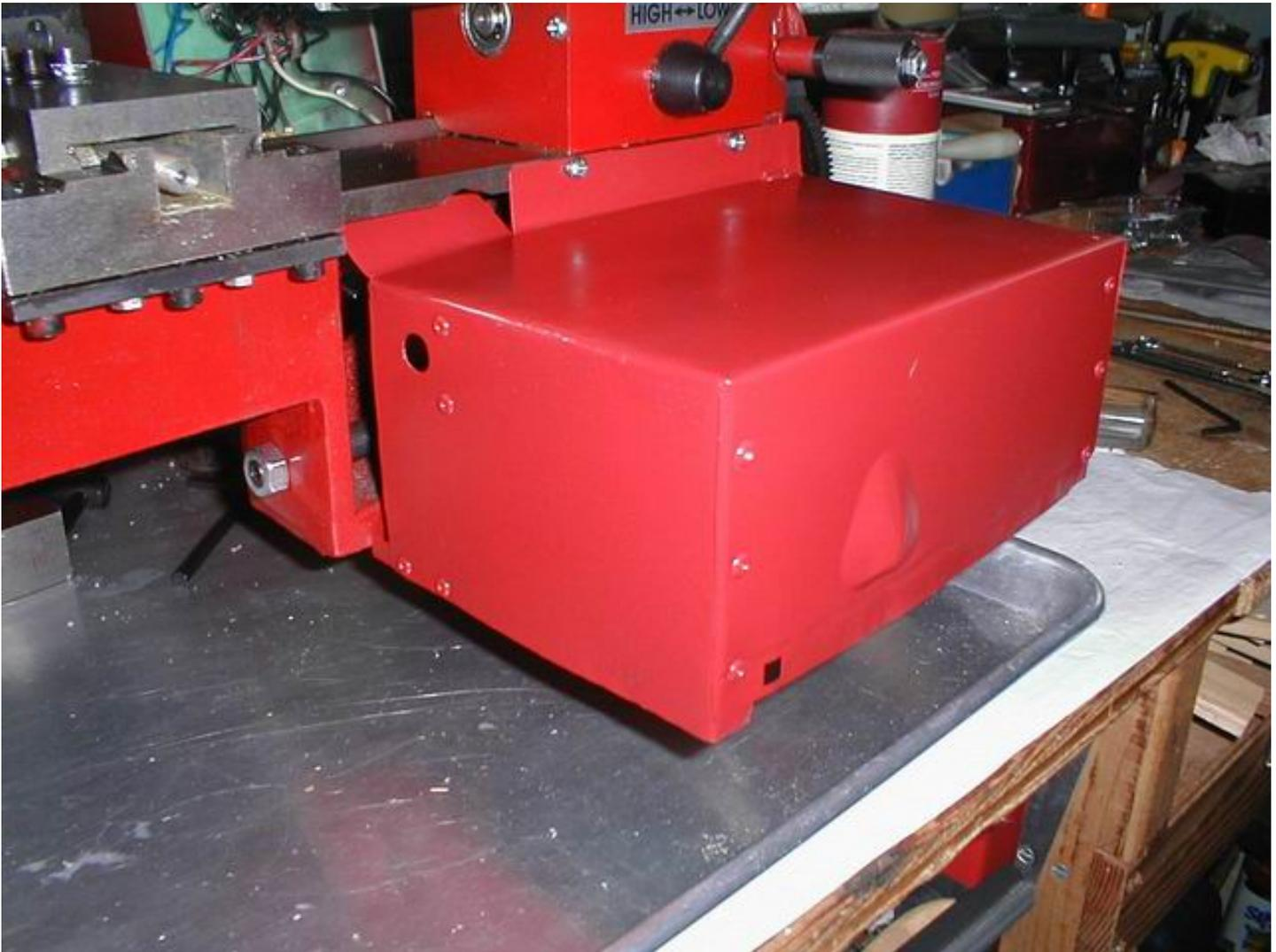
Coupled with adjustments made to the three potentiometers on the controller board, this lathe modification (which requires no changes to the original hardware, save the clamp from the old motor cover) has greatly expanded the versatility of the machine, provides lots of torque at the slowest speeds and runs fast enough for all the jobs we have experienced.
